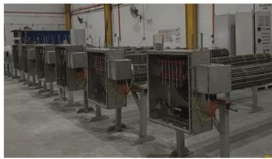
Immersion heating is used to heat up and/or maintain the medium in the tank for application such as bitumen, crude oil, condensate, or CIP use in Seawater Treatment.
