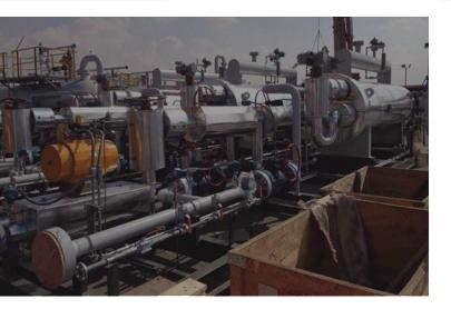
This relates to cryogenic applications where the heater will heat the very low-temperature liquid and vaporise it. The vaporised gas can then be further heated by a gas heater in the second stage of heating to the desired temperature.
